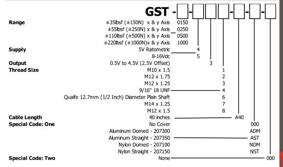
The KA configuration tool is used to specify a standard KA Sensor, other options are available.
